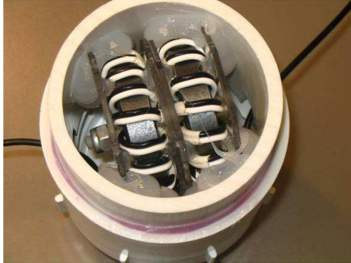
**Figure 3: The 4:1 Current Balun - Inside View of Toroid Cores with Windings**
