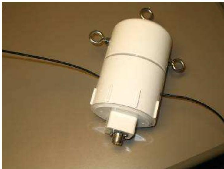
**Figure 4: Current Balun - Sealed and Ready for Installation**
